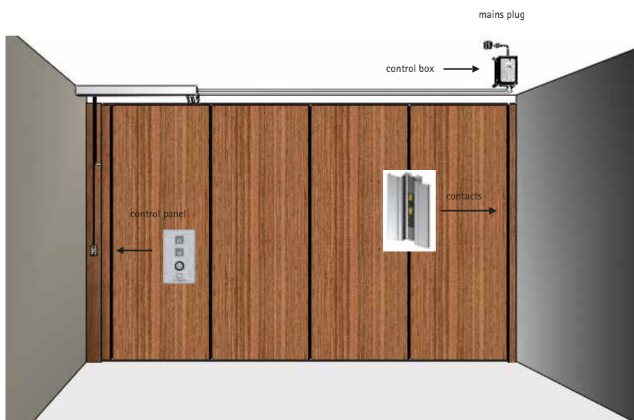
Pic. 7: Movable wall – semiautomatic operating system
