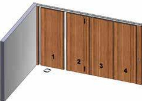
Pic. 8: Example of the opening procedure of panels with a single point suspension system.
